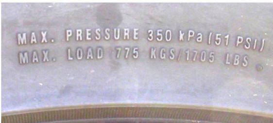
**Tyre Side-wall, showing Load Rating
