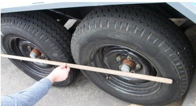
**Check Wheel-nuts and Alignment (tandem-axles)**
