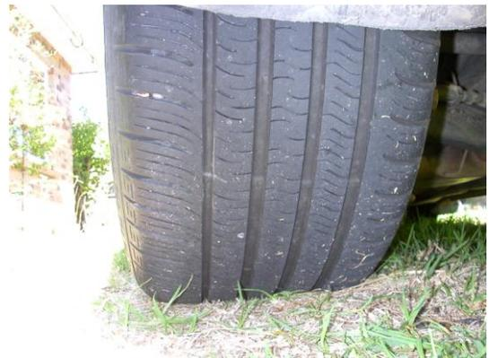
**Inspect Tyre Treads for wear or damage**
